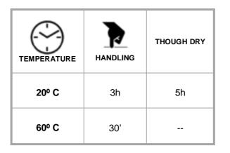
The product reaches its maximum performance after 15 days of drying in the air (ambient temperature 18-22°C) or in a shorter time at a higher temperature.
